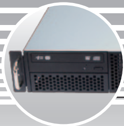
Flexible 5.25" ODD cage for different configuration
